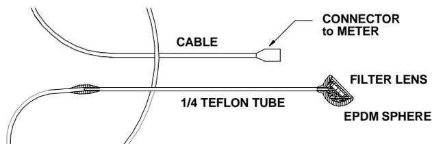
Cavitation generated by the sound pressure waves is produced in the form of bubbles that grow and implode with micro-streaming water jets hitting the filter surface. The sensor mounted behind the lens detects these impacts and the signal is sent via the cable to the electronic case.
