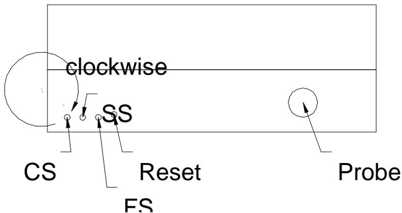
Ultrasonic cavitation energy meters have a **calibration screw (CS)** located on the top of the meter behind the receptacle for the ultrasonic probe. The location of the screw is shown on the drawing on the previous page. The **SS** and **FS** screws are disabled on the pb-500 meter. The procedure to calibrate the energy with this adjustment is as follows:
