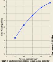
Chart 1: Cavitation meter readings versus applied generator power.
