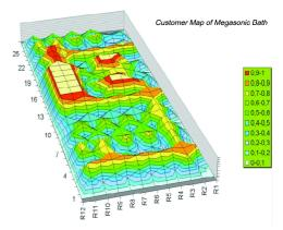
Figure 3: Mapping of a megasonic bath using the cavitation meter.
